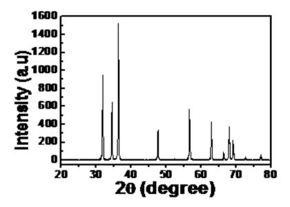
Fig.1 XRD pattern of Nanocrystalline ZnO QDs.
