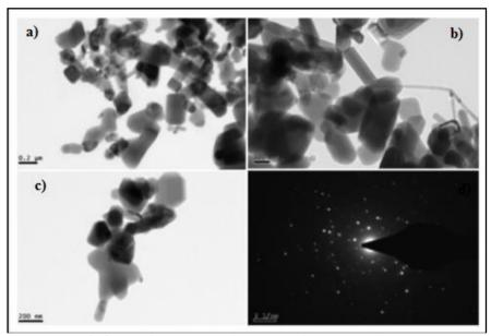
Fig.2 Transfer Electron Microscopy of Nanocrystalline ZnO QDs.
