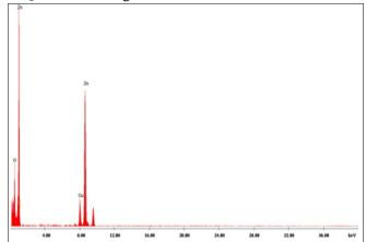
Fig. 4 Energy dispersive X-ray spectroscopy spectrum of ZnO Quantum Dots.
