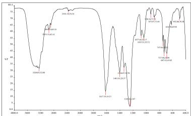
Fig.3. Fourier Transform Infrared Radiation Measurement Nanocrystalline ZnO QDs.
