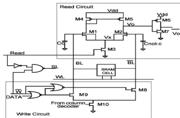
Figure 1: Proposed adiabatic SRAM cell design
