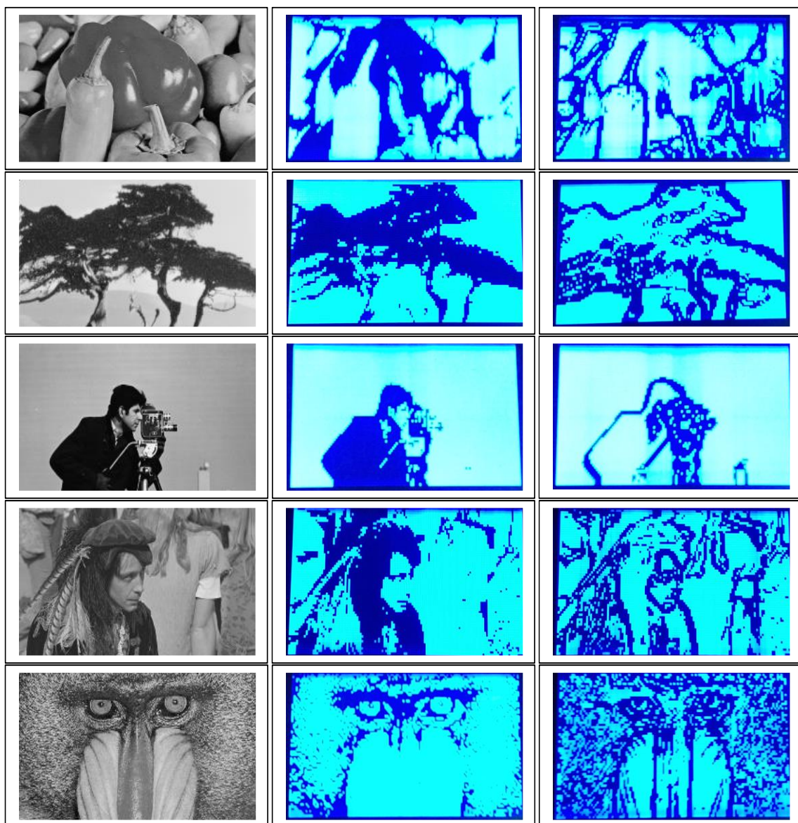
Figure 9: The first column represents the original images, the second column represents the original images displayed in the graphic LCD, the third column represents the image edges detected using Sobel detector displayed in the graphic LCD based on our system
